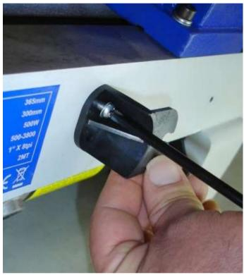
Attach the two cable tidy brackets with the four M5 x 12mm screws and washers provided.
