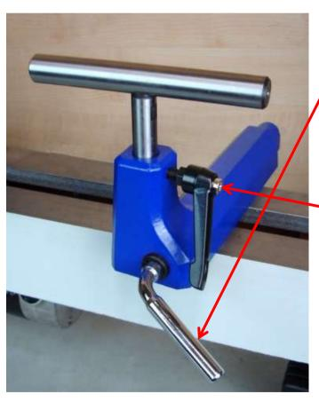
The tool rest can be moved along the bed of the lathe.
