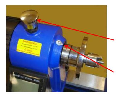
The lathe is fitted with an indexing system which allows the spindle to be locked in 24 positions (15 degree intervals)
