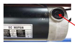
The carbon brushes should be regularly inspected and will need changing after approximately 500 hours use, or when the block has worn down to a length of 7mm.
