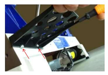
Using a cross-headed screwdriver, loosen the two screws in the rear of the lathe bed and attach the tool tray, ensuring the washers are positioned next to the screw head. Re-tighten the screws.
