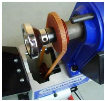
2) Open the upper belt cover which is hinged at the bottom.
