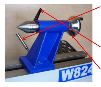
To slide the tailstock along the bed, pull up the silver tailstock locking lever.
