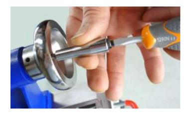
Using a flat bladed screwdriver, attach the handle to the tailstock hand wheel.
