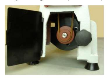
The lathe has electronic speed control. There are two ranges of speeds which are obtained by changing the position of the drive belt.
