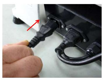
Connect the Power Cord to the socket in the rear of the Speed Control Box.
